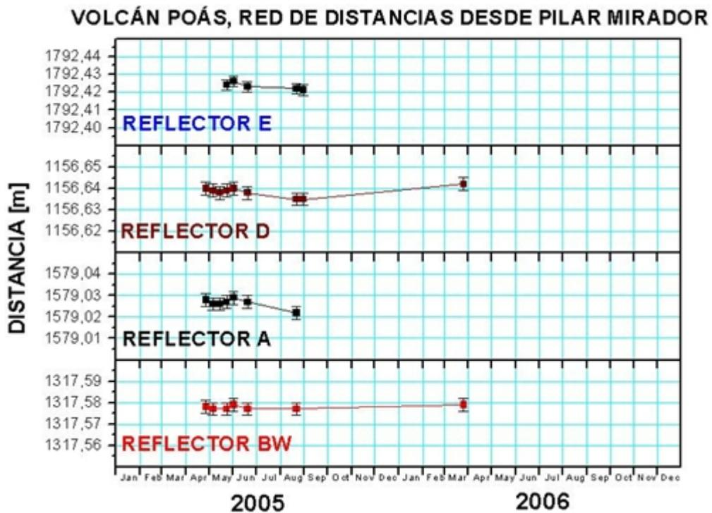
Figure 14: Inclined distances across the main crater of Poas measured from a pillar to fixed reflectors. This figure shows error bars that represent the typical dispersion of 3 mm present in these measurements.
