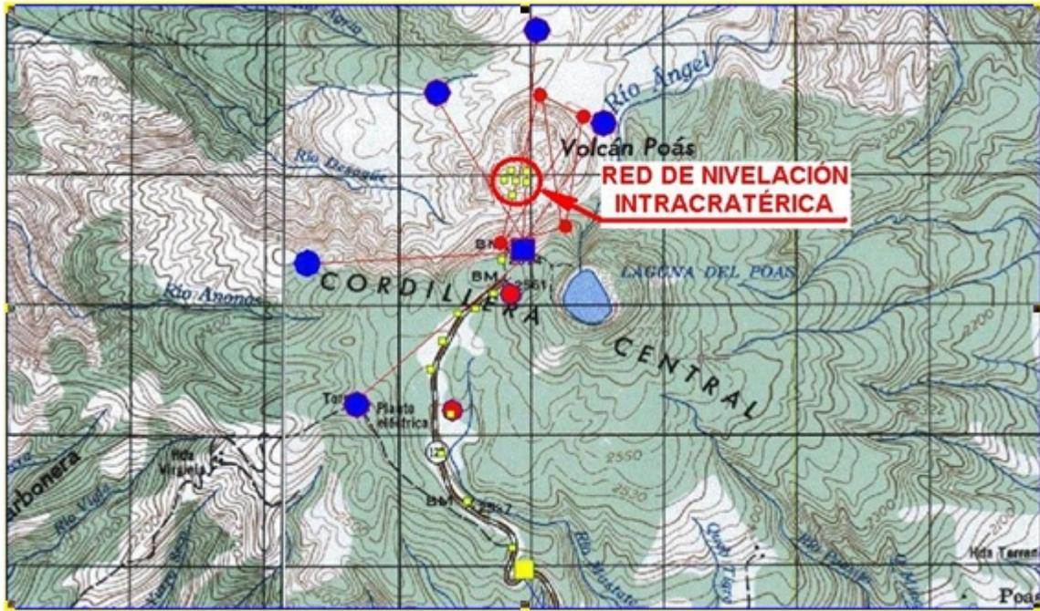
Figure 13: Deformation network for Poas volcano. The blue square is the pillar and the blue circles are the fixed reflectors.
