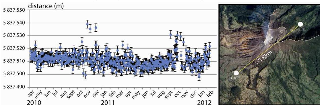
Figure 6: Distance time series between the 2 permanent GPS stations CAPI (southwest of the volcano) and GIBE (northeast of the volcano)
