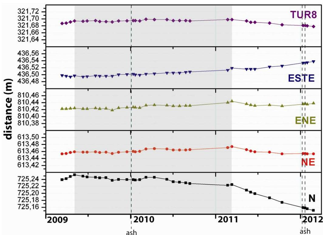
Figure 5: Electronic Distance Measurements between the overlook and various prisms (Fig. a) since early 2009.
