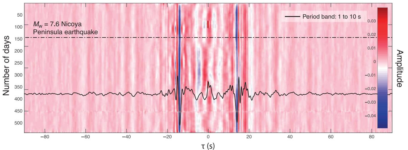
**Fig. 2. Cross-correlation of ambient seismic noise.** Daily GFs filtered between 1 and 10 s for the station pair INDI-SAJU. The black trace represents the reference GF (RGF). The dotted line indicates the time of the Nicoya Peninsula earthquake. Note the high symmetry between the causal and acausal signals.
