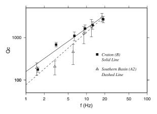
**Fig. 8** Plot of  $Q_c \times f$  (Hz) for craton stations (group B) and southern part of the Parecis basin (subgroup A2) for window length of 45 s
