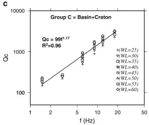
**▼ Fig. 7**  $Q_c(f)$  for all data groups with fitted relationship  $Q_c = Q_0 f^{\eta}$ . Data points refer to the eight windows lengths (WL). **a** Group A (stations in the basin); **b** group B (stations in the cratonic basement),  $Q_c = 167 f^{1.03}$ ; and **c** group C (all stations of both networks),  $Q_c = 99 f^{1.17}$ .  $R^2$  is the correlation coefficient
