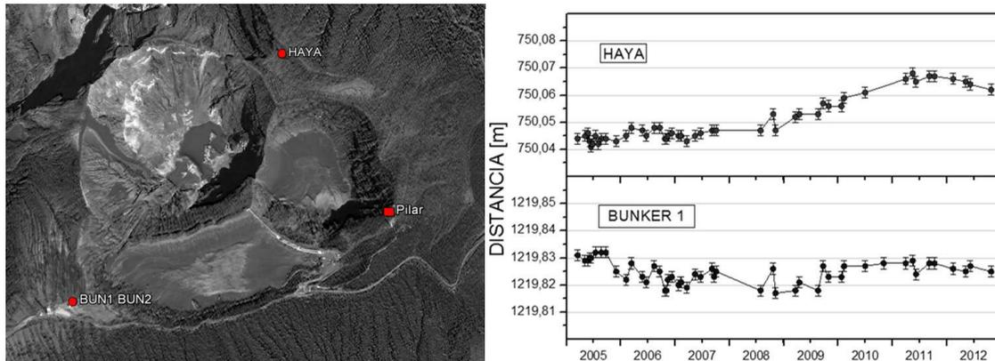
Figure 14: a) EDM Network at Irazú volcano (BUN1, BUN2, HAYA), measured from Pilar. b) Longitude lines of EDM, observed from Pilar at the summit of Irazú volcano.
