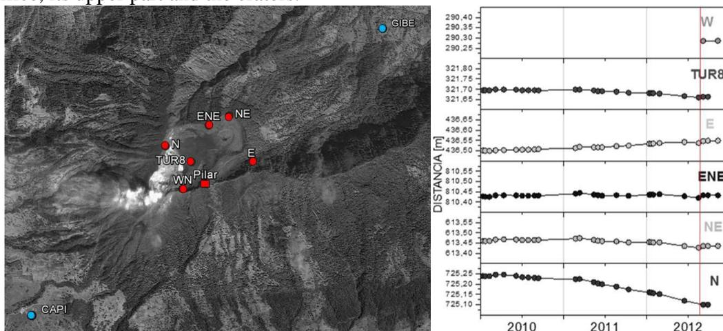
Figure 5: a) Geodesic network of Turrialba volcano in 2012. Red circles: reflectors of the EDM network measured from the Pilar (red square). Blue circles: permanent GPS stations (CAPI and GIBE). b) Longitudes of the EDM lines as defined Fig.5a. in 2010-2012. The red line marks the Mw 7.6 earthquake of Nicoya on September 5<sup>th</sup>, 2012. Generally a contraction of the distances is noticed in 2012.
