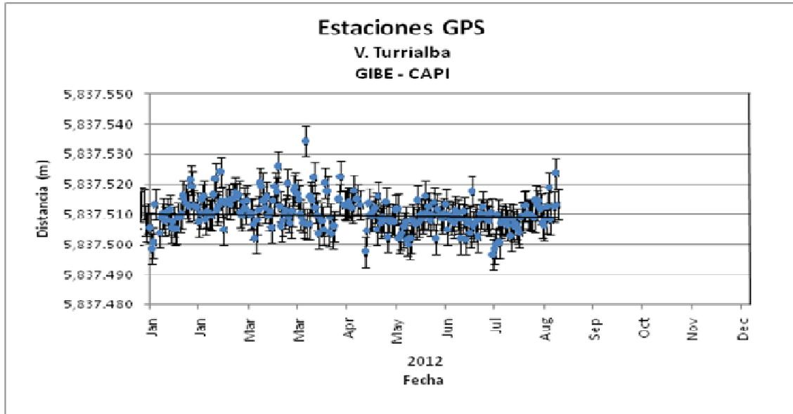
Figure 6: Geometrical distance between the 2 permanent GPS stations CAPI and GIBE for 2012.
