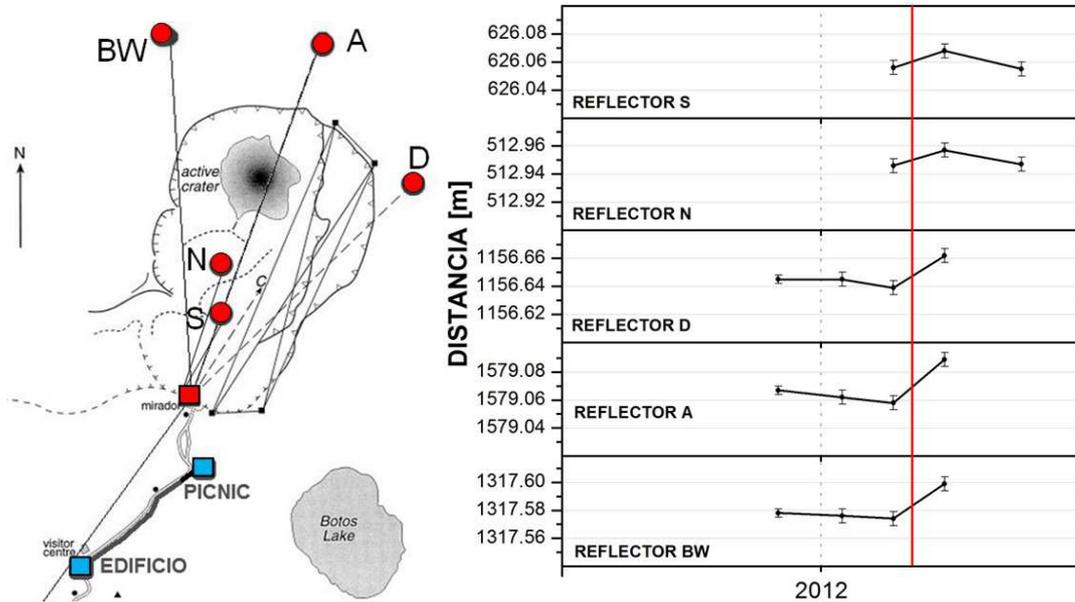
Figure 19: a) Geodesic network at Poás volcano. Red circles: EDM reflectors for which the distance is measured from the Pilar (red square). In blue are the 2 marks of the geometrical leveling. b) Longitude lines of the EDM network, observed from the Pilar at the Mirador of Poás volcano. A contraction was generally observed until the September 5<sup>th</sup> Nicoya earthquake. The S and N reflectors present the same tendency after this tectonic event.
