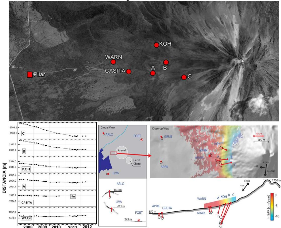
Figure 24: a) The geodesic network at Arenal volcano in 2012. Red circles: EDM network measured from Pilar. b) EDM results for the west flank of the volcano. c) Calculation of speed of deformation between 2008 and 2009 using EDM, GPS and 2005-2009 InSar techniques (Muller et al., 2011).
