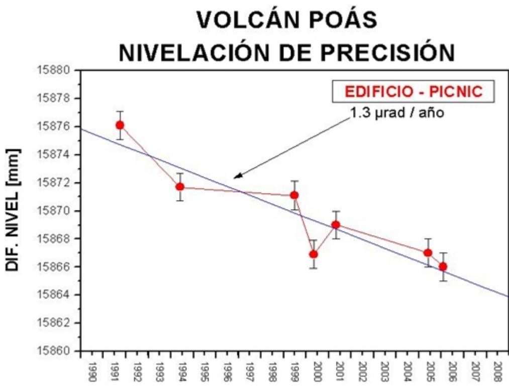
Figure 15: Changes in elevation of the radial line between the Picnic area and the Nacional Park building using trigonometric leveling.
