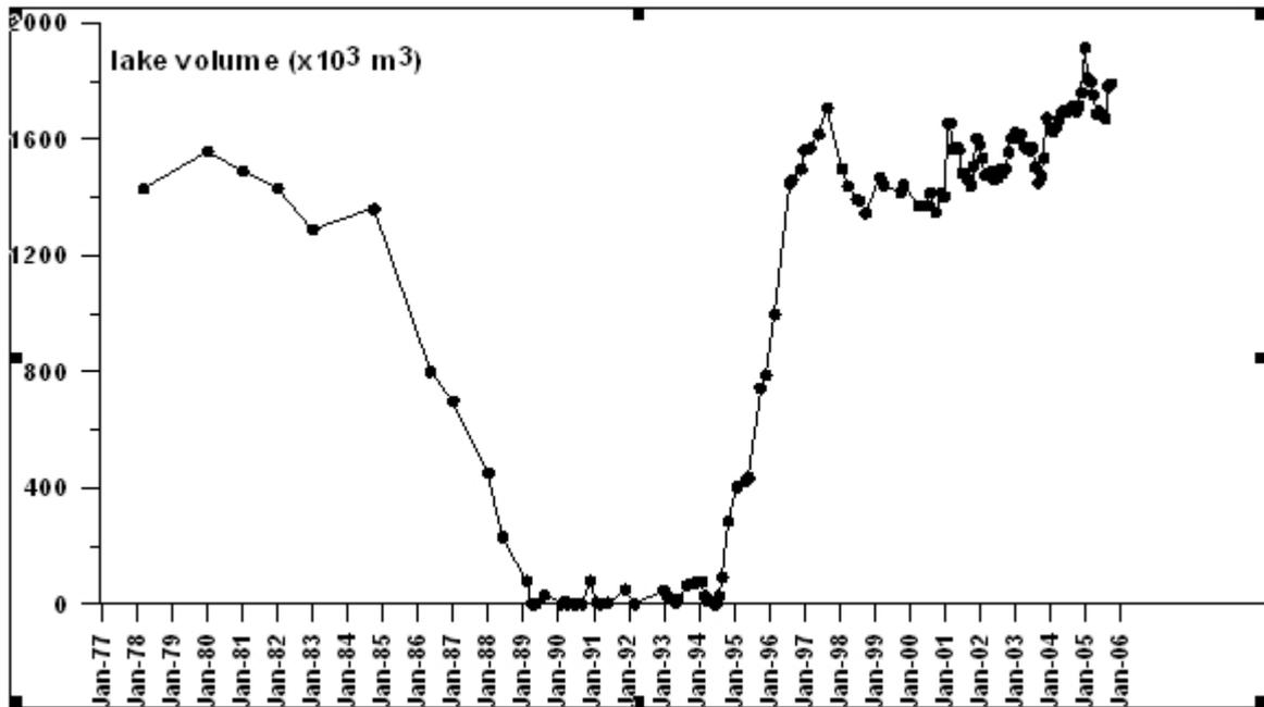
Figure 6: Variations in the volume of Laguna Caliente, Poas main crater lake, 1977-2006. Depth of the lake was about 45 m in late 2005. Notice that the lake increased its temperature from 51 °C by February, 28, 2006 to 54 °C by April 01, 2006, but in contrast, the lake pH reached a minimum of 0.59 by February 28, 2006, This pH increased to 0.65 by April 01, 2006 and 0.71 by April 06, 2006.
