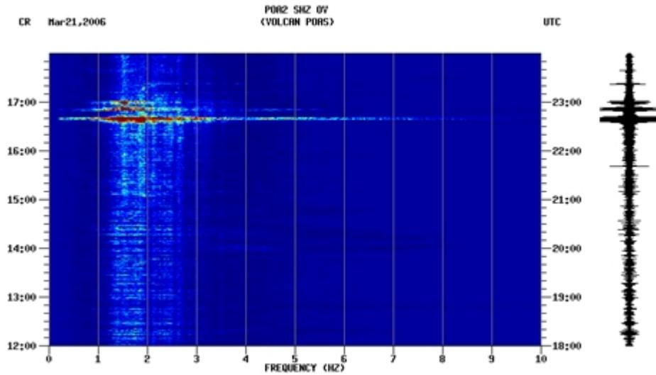
Figure 8: Signal and spectrogram of the seal rupture signal recorded March 21, 2006 at 22:19 hrs GMT.
