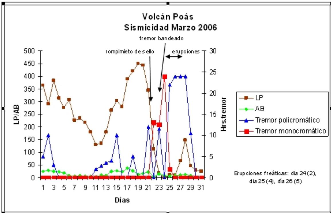
Figure 7: Seismicity of Poas volcano during March, 2006 based on records from the POA2 seismic station of OVSICORI-UNA.
