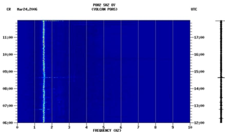
Figure 10: Seismic signal and spectrogram corresponding to the first phreatic eruption occurred at 17:57 hrs GMT, March 24, 2006. The seismic signal in the spectrogram is located in the upper part of the spectrogram with a dominant frequency of 2.8 Hz. The dominant frequency in the rest of the spectrogram corresponds to the monochromatic harmonic tremor.
